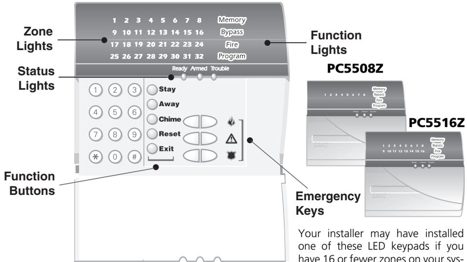
Your installer may have installed one of these LED keypads if you have 16 or fewer zones on your system. These keypads operate in the same way as the PC5532 keypad.
